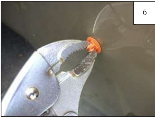
Remove two clips from front using vise grips, pulling with a rocking motion. See step 7.
